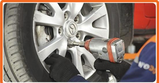
Lower the car and working in a cross order, tighten the wheel bolts.
