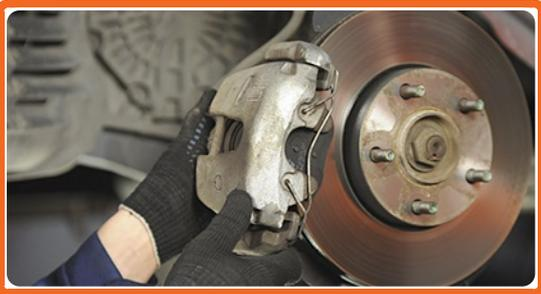
Remove the brake caliper.
