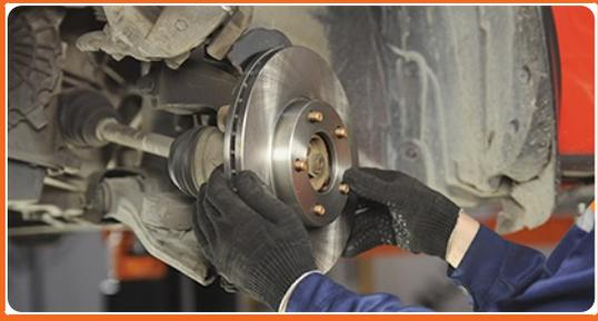
Install the new brake disc on the hub and tighten the screws.
