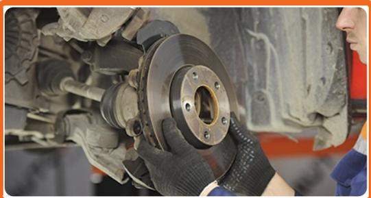
Unscrew the brake disc mounting bolts and remove it.
