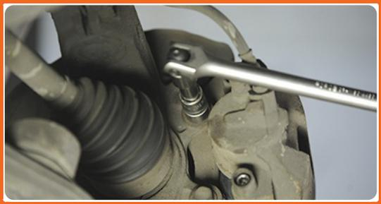
Unscrew the brake caliper fastening
