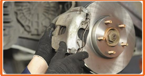
Install the brake caliper and fix it.
