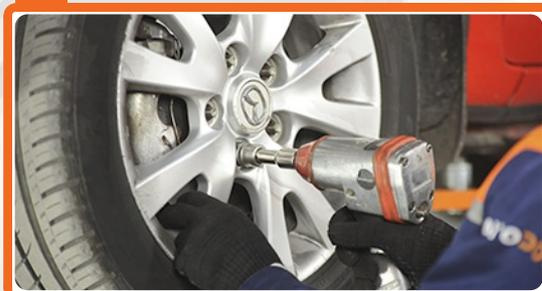
Loosen wheel bolts on standing on the ground vehicle
